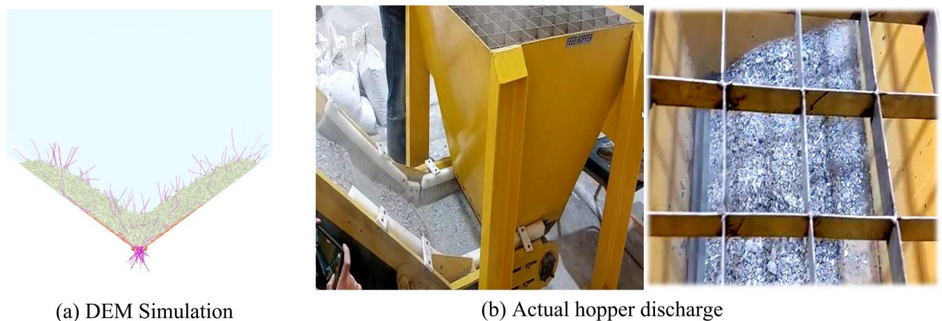
Figure 4. Hopper discharge system: (a) DEM simulation of mixed-particle flow behavior; (b) experimental validation of actual hopper discharge operation with grid-type outlet configuration. A DEM simulation video of the optimal hopper discharge is provided in Supplementary Video S1.
