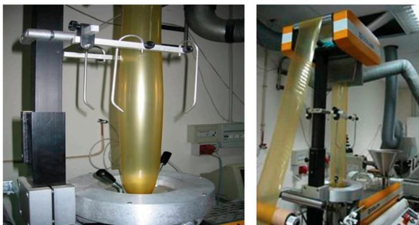
**Figure 2.** Lab-scale film blowing of thermoplastic zein. Reproduced with permission from [91]. Copyright publisher, 2020. In the figure, the film bubble during the film-blowing process of thermoplastic zein is shown. The zein powder was first plasticized with poly (ethylene glycol) 400 directly in the extruder, without the use of a solvent and of a premixing phase.
