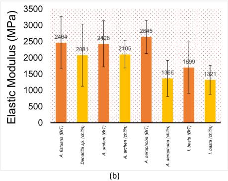
**Figure 5.** Elastic modulus (nanoindentation) in megapascals (MPa) of (a) 10  $\mu$ m sections; (b) 1  $\mu$ m sections of selected demosponges under study (from left to right: *A. fistularis, Dendrilla* sp., *A. archeri, A. aerophoba, Ianthella basta*)  $\pm$  standard deviation. "BrT" denotes bromotyrosine-containing (orange). "Chitin" denotes sponge samples where bromotyrosines have been chemically removed (yellow).
