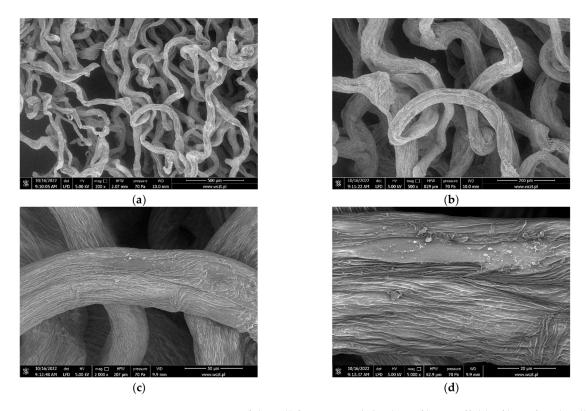
**Figure 8.** SEM images of the cell-free *A. aerophoba* chitin fibre scaffold's fibre after decellularisation (a)  $\times 200$ ,  $500 \, \mu m$ ; (b)  $\times 500$ ,  $200 \, \mu m$ ; (c)  $\times 2000$ ,  $50 \, \mu m$ ; and (d)  $\times 5000$ ,  $20 \, \mu m$ .
