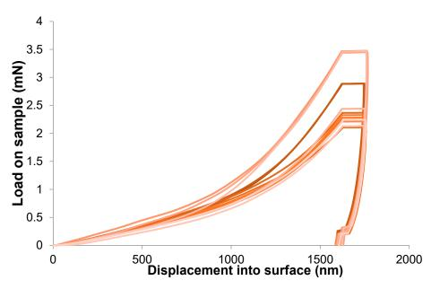
**Figure 7.** Indentation hysteresis curves for measurements on chitinous fibres of *A. aerophoba* demosponge origin.
