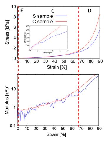
**Figure 2.** Stress–strain and modulus–strain curves of the investigated *A. aerophoba* sponge scaffolds. Three distinctive stages of compression were indicated: E—elastic stage, C—collapse stage, and D—densification stage. S samples (blue) correspond to bromotyrosine-containing samples and C (red) corresponds to bromotyrosine-free samples.
