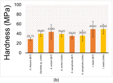
**Figure 6.** Hardness (nanoindentation) in megapascals (MPa) of (a) 10  $\mu$ m sections; (b) 1  $\mu$ m sections of selected decellularised fibres (from left to right: *A. fistularis, Dendrilla* sp., *A. archeri, A. aerophoba, I. basta*)  $\pm$  standard deviation. "BrT" denotes bromotyrosine-containing (orange). "Chitin" denotes sponge samples where bromotyrosines have been chemically removed (yellow).
