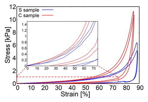
**Figure 4.** Loading–unloading hysteresis curves of the investigated chitinous scaffolds isolated from *A. aerophoba* demosponge. S samples (bromotyrosine-containing, blue), C samples (bromotyrosine-free, red).
