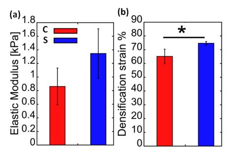
**Figure 3.** Comparison of elastic modulus (**a**) (compression) (MPa) and (**b**) densification strain (%) of bromotyrosine-containing (S, blue) and bromotyrosine-free (C, red) chitinous scaffolds isolated from *A. aerophoba* demosponge. \* p < 0.05.
