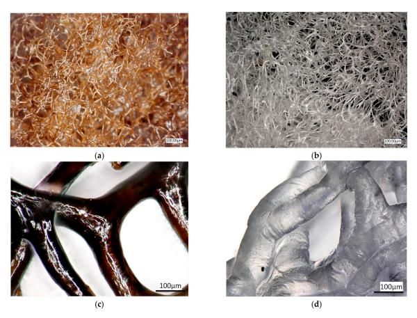
**Figure 9.** Digital microscopy images of the *A. aerophoba* chitin fibre scaffold after decellularisation. (**a**,**c**) Bromotyrosine-containing chitin scaffold, featuring a 3D porous network of microfibers. (**b**,**d**) Bromotyrosine-free chitin scaffold, featuring the same 3D porous network of microfibers.
