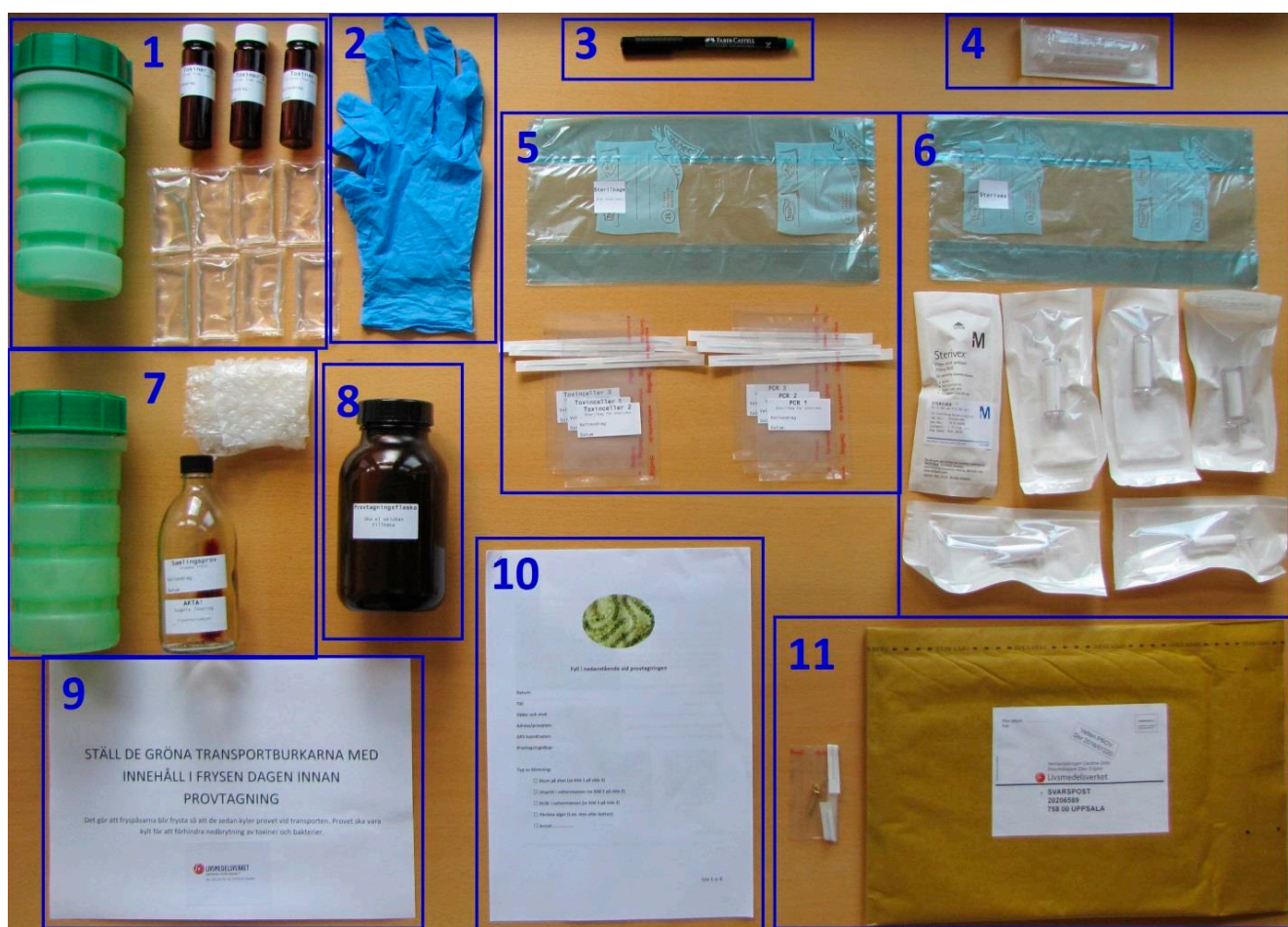
Figure 4. Cyanobloom sampling kit: (1) green transport container with 7–8 freezer bags and three brown filtrate bottles labeled “Toxins 1–3”; (2) a pair of sampling gloves; (3) a permanent marker; (4) a syringe; (5) freezer bag, marked “Steribag/For Sterivex” containing 3 sterile bags marked “Toxin cells 1–3” and 3 sterile bags marked “PCR 1–3”; (6) freezer bag, labeled “Sterivex” containing 6 Sterivex filters; (7) green transport container with “Sample collecting bottle” with 1 mL of Lugol’s solution and bubble wrap for transport; (8) large sampling bottle, amber; (9) sheet with the information to place the kit in the freezer the day before sampling; (10) algal bloom sampling protocol; and (11) padded return envelope with the accessories for closure.
