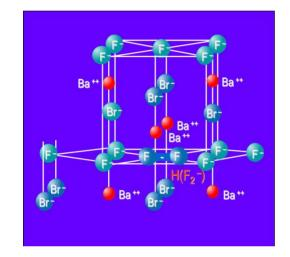
**Figure 13.** Model of the BaFBr lattice cell with  $H(F_2)$  center.
