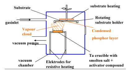
A crystalline layer of phosphor is deposited on the substrate. In a certain pressure and substrate temperature range, phosphor crystals grow as needles, perpendicular to the substrate surface [55-57] (Figure 20).
