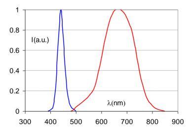
The short  $Eu^{2+}$  characteristic decay-time makes fast read-out possible and the material has a convenient stimulation spectrum maximum at 680 nm.
