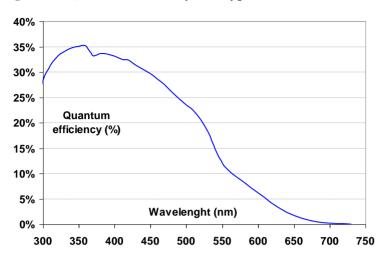
Figure 5. Quantum efficiency of a typical CR scanner PMT.
