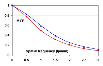
Thanks to the much higher X-ray absorption, however, NIP improved the DQE by a factor of 2 at low spatial frequencies and by up to a factor 5 for the higher spatial frequencies (>3 lp/mm) with respect to PIP (Figure 35). It was confirmed in this study that, for general radiography, CR with NIP would be able to match the technical image quality obtained with DR based on CsI:Tl<sup>+</sup> needle plates and amorphous Si photo detectors.
