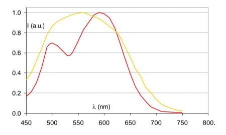
**Figure 15.** Stimulation spectrum measured at 300 K after X-ray exposure of  $Ba_{0.88}Sr_{0.12}F_{1.09}Br_{0.91}$ : Eu<sup>2+</sup> (**a**), and after erasure and 2 (**b**), 4 (**c**) and 8 (**d**) h replenishment.
