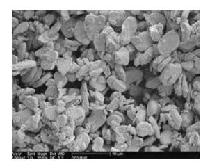
**Figure 6.** SEM image of BaFBr:Eu<sup>2+</sup> storage phosphor powder.
