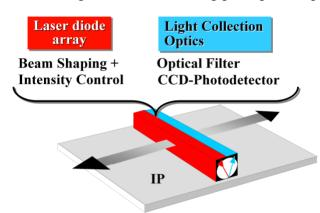
Figure 22. Schematic diagram of line-scanning principle (adapted from [77]).
