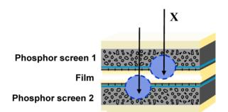
Figure 1. Screen / film detector, used in conventional radiography.
