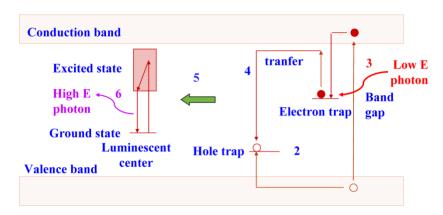
Figure 3. Energy diagram showing photo-stimulated luminescence in a storage phosphor.
