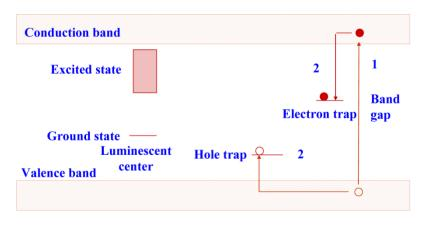
Figure 2. Energy diagram showing electron and hole trapping in a storage phosphor.
