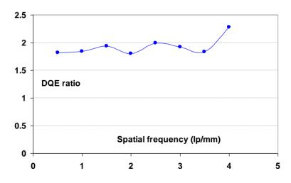
A thorough analysis was done of the improvement in technical image quality of  $DX-S^{\text{(B)}}$  with NIP with respect to a PIP based CR system [111]. The conclusion was that the higher DQE of  $DX-S^{\text{(B)}}$  is not
