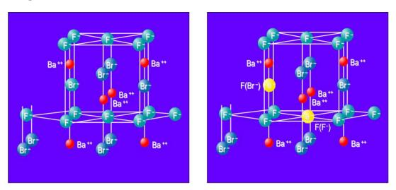
**Figure 9.** Model of the BaFBr lattice cell (**a**) with  $F(Br^{-})$  and  $F(F^{-})$  centers (**b**).
