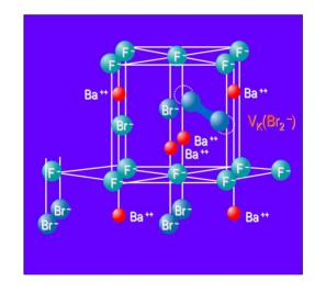
**Figure 10.** Model of the BaFBr lattice cell with  $V_K$  (Br<sub>2</sub><sup>-</sup>) center.
