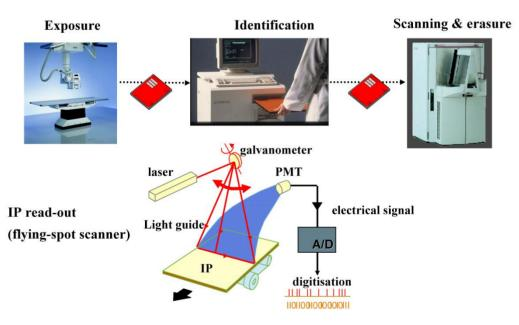
Figure 4. CR storage phosphor plate exposure and read-out.
