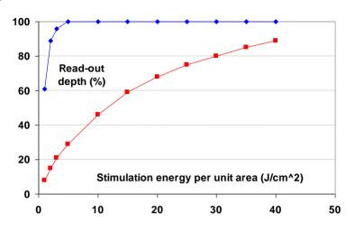
The stimulation energy is only 4  $\mu$ J/mm<sup>2</sup> as for CsBr:Ga<sup>+</sup>. CsBr:Eu<sup>2+</sup> needle imaging plates have been introduced for general radiography by Agfa in 2005. More recently, NIP's became available for mammography as well [80].
