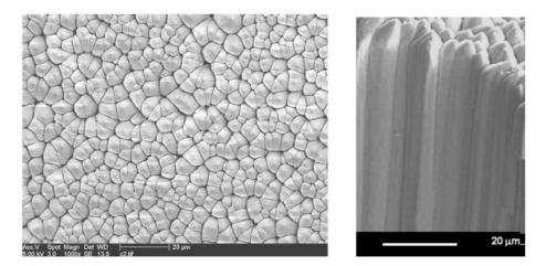
Since materials for vapor deposition must melt congruently (without decomposition), needle phosphors are mostly chemically simple compounds, containing 1 anion and 1 cation.
