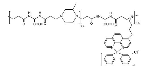
Figure 24. Poly(amidoamine) Ir(III) complex as a new <sup>1</sup>O<sub>2</sub> sensitizer.
