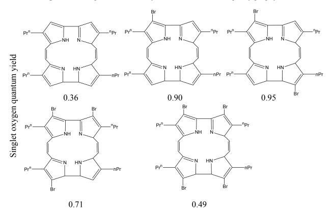
Figure 22. Brominated porphycene macrocycles and their <sup>1</sup>O<sub>2</sub> quantum efficiency.
