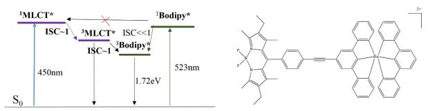
**Figure 32.** Energy diagram for a Ru(II) complex having BODIPY as a visible light harvesting ligand, showing energy transfer is unlikely.
