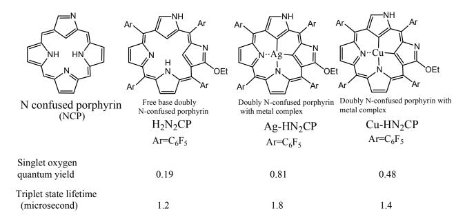
Figure 17. Properties of N-confused porphyrin (H<sub>2</sub>N<sub>2</sub>CP) with, and without, metal atoms.
