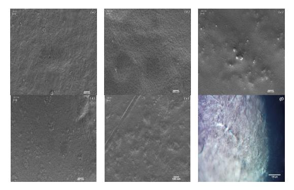
**Figure 1.** Scanning electron microscopy (SEM) micrographs of the composite films containing (**a**) 0, (**b**) 1, (**c**) 2, (**d**) 3 and (**e**) 4 wt % diamond nanoparticles. The scale bar is 300 nm. (**f**) Transmission optical micrographs of chitosan/bacterial cellulose (CS/BC) film.
