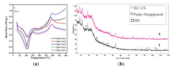
**Figure 4.** (a) Differential scanning calorimetric traces of CS/BC composite films containing different amounts of NDs. (b) X-ray diffraction (XRD) pattern of (1) CS/BC and (2) CS/BC/ND (4wt%). Note the disappearance of the green circles and the appearance of purple squares after ND addition.
