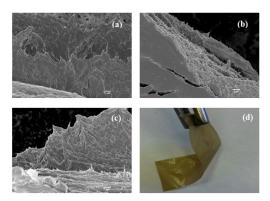
**Figure 5.** SEM images show the fracture surface of CS/BC films containing (wt %) (**a**) 0, (**b**) 2 and (**c**) 4 NDs. (**d**) Digital image illustrates the flexibility of the nanocomposite films.
