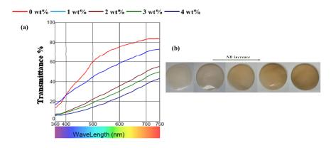
Figure 3. (a) Transmission profile of composite films containing different amounts of ND.(b) Digital images show the appearance of the composite films.
