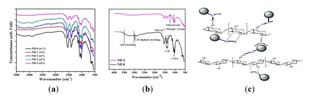
**Figure 2.** (**a**,**b**) Fourier transform infrared (FTIR) spectra of composite films. (**c**) Schematic illustration of possible interactions between the polymer matrix and functional groups of NDs.
