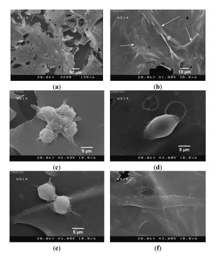
Figure 7. Representative SEM images of composite films. The films were prepared by freeze drying. (a) The film surface before cell incubation shows the porous structure of the freeze-dried specimen. Cell morphology on  $(\mathbf{b},\mathbf{c})$  CS/BC and  $(\mathbf{d}-\mathbf{f})$  CS/BC/ND (4 wt %) films.
