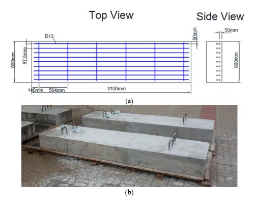
**Figure 5.** Concrete wide beam test specimen. (a) The planar and side views; (b) the test specimen after casting.
