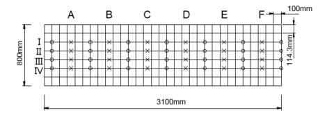
**Figure 10.** A planar view of the  $114 \times 100 \text{ mm}^2$  test point grid for P-wave measurements. The test was carried out on the grid locations. The O and X marks indicate the positions of the transducers and average measurements, respectively. All dimensions in millimeters.
