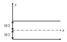
Figure 1. Schematic geometry of a free plate problem with regard to the Lamb wave.
