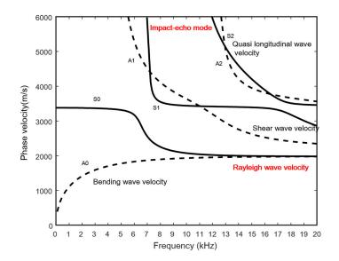
**Figure 3.** Phase velocity dispersion curves determined by MASW (based on the FE simulation of a concrete slab with a thickness of 0.3 m). A density of 2250 kg/m<sup>3</sup>, an elasticity of 23 GPa and a fixed Poisson's ratio of 0.167 are assumed for the concrete slab.
