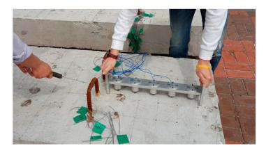
**Figure 7.** The MDAFS testing configuration for the MASW along predefined paths on the surface of a concrete wide beam.
