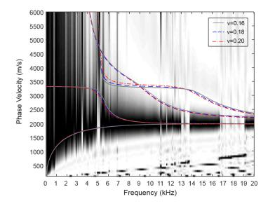
**Figure 12.** The theoretical dispersion curves on the experimental dispersion spectrum for three values of Poisson's ratios in the W2 concrete wide beam.
