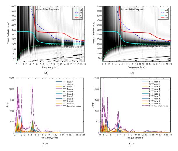
**Figure 11.** Experimental MASW results for two concrete wide beams (W2 and W4). A Poisson's ratio of 0.16 was measured for the concrete cylinder. (**a**) Phase velocity dispersion curve along path III in the W2 beam; (**b**) summed amplitude spectra along path III in the W2 beam; (**c**) phase velocity dispersion curve along path II in the W4 beam: (**d**) summed amplitude spectra along path II in the W4 beam.
