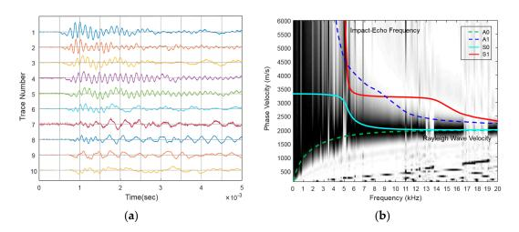
**Figure 8.** Experimental MASW results along Path III in specimen W2. The computed A0, A1, S0 and S1 Lamb modes corresponding to the specimen depth overlap on the dispersion curve image. (**a**) The signals in the time domain; (**b**) dispersion curve.
