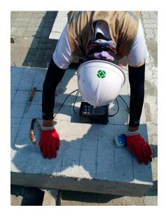
Figure 9. P-wave measurement in a grid on the surface of a concrete wide beam.
