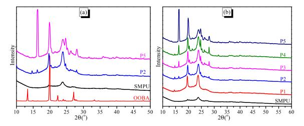
**Figure 3.** WAXD patterns of the samples (**a**) OOBA, SMPU, P2 and P5; (**b**) SMPU and SMPU-OOBAm composites with various OOBA contents.
