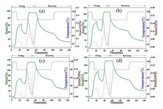
**Figure 11.** Strain-time-temperature curves showing triple shape memory effects for (**a**) P1; (**b**) P2; (**c**) P3 and (**d**) P4.
