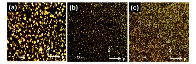
**Figure 10.** POM images of (**a**) P2 at 86 °C; (**b**) P4 at 95 °C; (**c**) P5 at 95 °C. ( $400 \times$ ) A: analyzer and P: polarizer.
