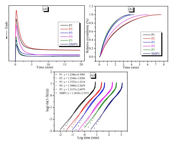
**Figure 6.** Isothermal crystallization behaviors of the SMPU-OOBAm composites. (**a**) Exothermic curves versus time; (**b**) Dependency of relative crystallinity versus time; (**c**) plots of  $\log\{-\ln(1 - X(t))\}$  versus  $\log(t)$  and the fitting line at 137 °C.
