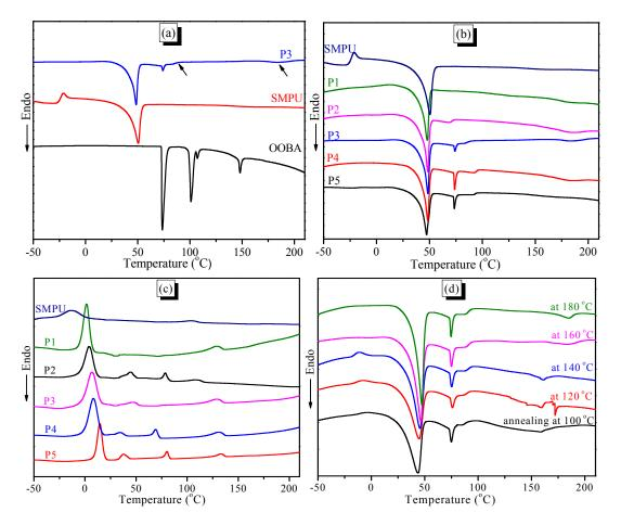
**Figure 5.** DSC curves of samples (**a**) OOBA, SMPU, and P3 on the second heating process; (**b**) SMPU-OOBAm composites on the second heating process; (**c**) SMPU-OOBAm composites on the cooling process; (**d**) P3 thermal treated at various annealing temperatures.
