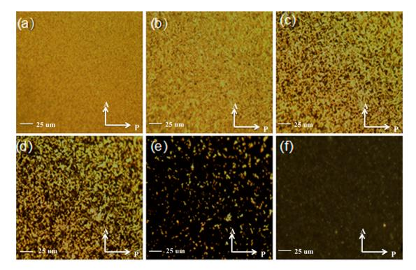
**Figure 9.** Representative POM images of P5 in the heating process ((a) 28 °C; (b) 59 °C; (c) 76 °C; (d) 95 °C; (e) 106 °C; (f) 180 °C). (400×) A: analyzer and P: polarizer.
