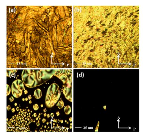
**Figure 8.** Representative POM images of pure OOBA upon heating (**a**) 50 °C; (**b**) 112 °C; (**c**) 135 °C; and (**d**) 139 °C. ( $400 \times$ ) A: analyzer and P: polarizer.
