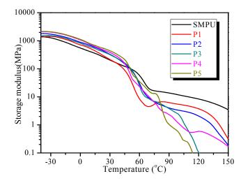
Figure 7. Storage modulus of SMPU-OOBAm composites.
