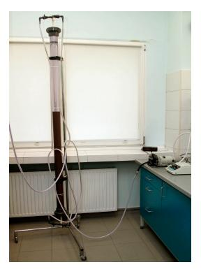
Figure 1. Ion-exchange column for the production of Ni(ReO<sub>4</sub>)<sub>2</sub>.
