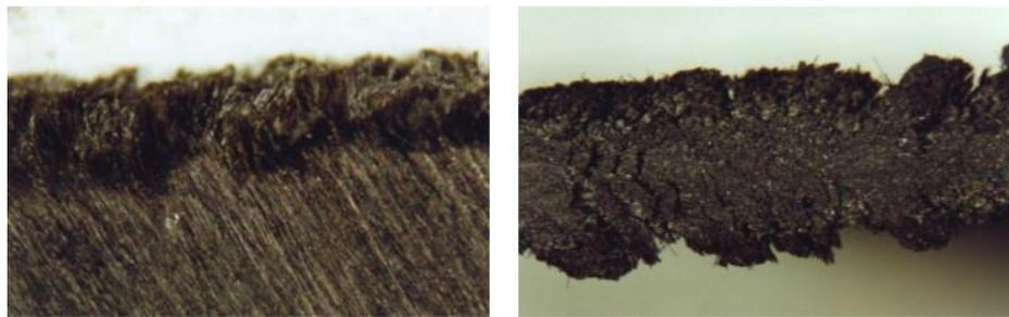
**Figure 3.** Damaged CFRP pultruded specimen trimmed with the V-shaped tool. Fibre orientation angle  $\theta = 120^\circ$  [62].
