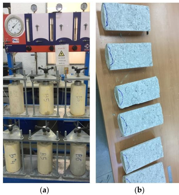
Figure 2. Depth of penetration of water under pressure (a) test and (b) specimens.
