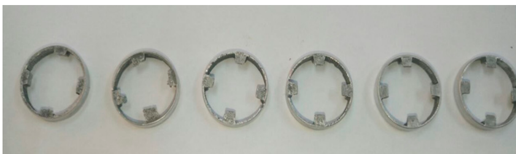
Figure 9. Spacer after long-term operation.
