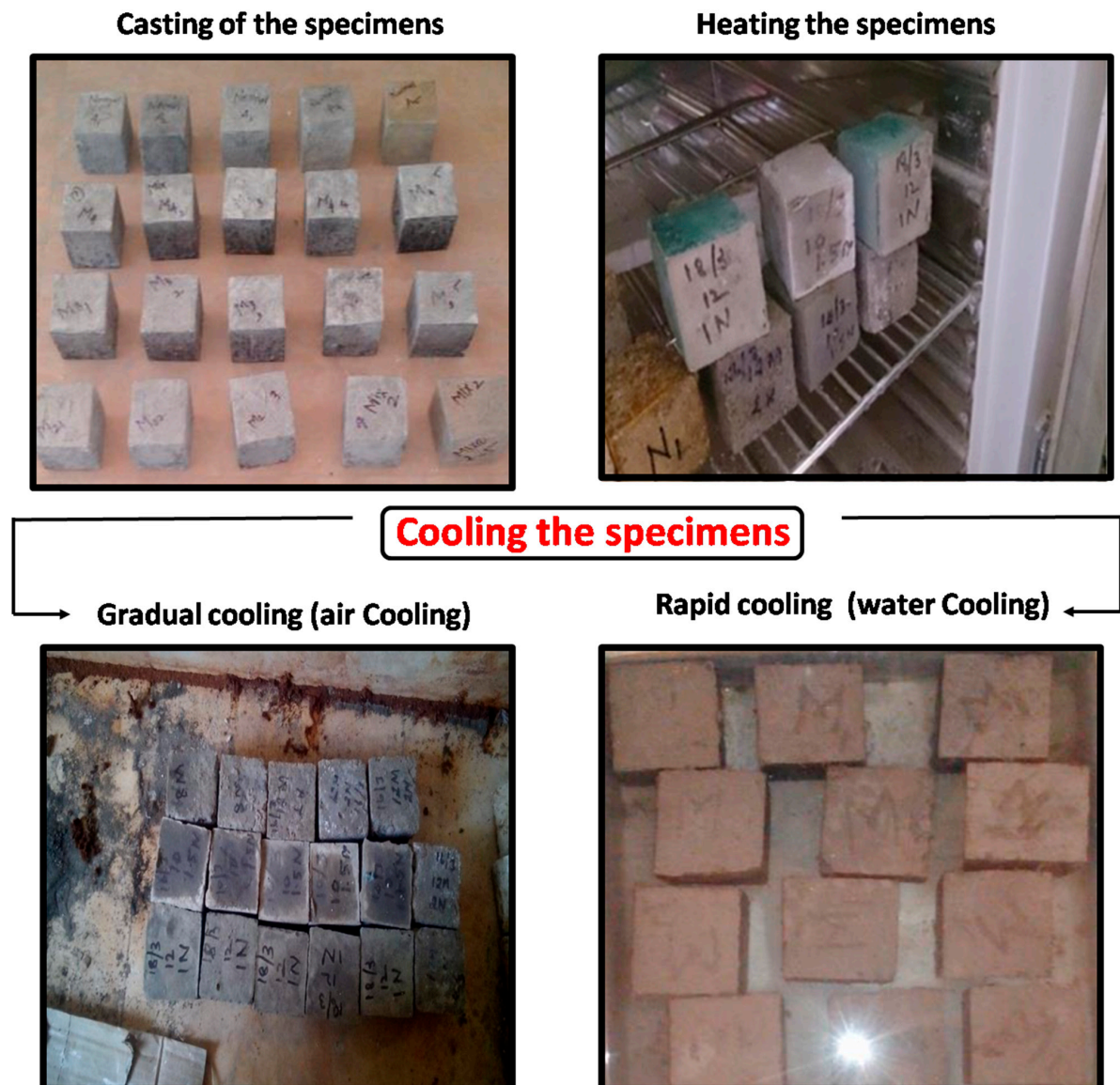
Figure 4. Self-compacting glass mortar specimens.
