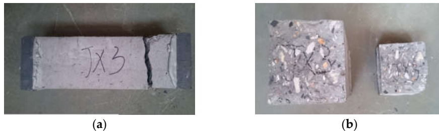
Figure 9. Failure modes of SCC prismatic specimens under cyclic direct tension. (a) Crack positions and (b) crack surfaces.
