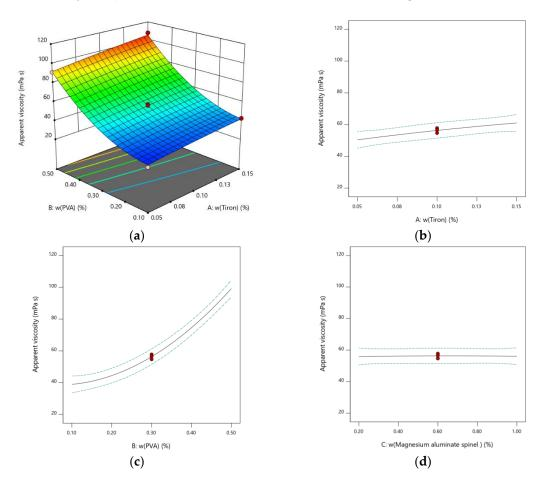
**Figure 2.** The effect on apparent viscosity of 70 wt.% Al<sub>2</sub>O<sub>3</sub> suspensions which contain 20 dwb.% waste Al<sub>2</sub>O<sub>3</sub> powder: (**a**) 3D-plot of viscosity on two factors (PVA content and Tiron content); (**b**) Tiron; (**c**) poly (vinyl alcohol) (PVA); (**d**) magnesium aluminate spinel (MgAl<sub>2</sub>O<sub>4</sub>).
