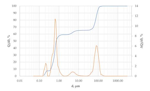
Figure A1. Particle size distribution for waste alumina powder.
