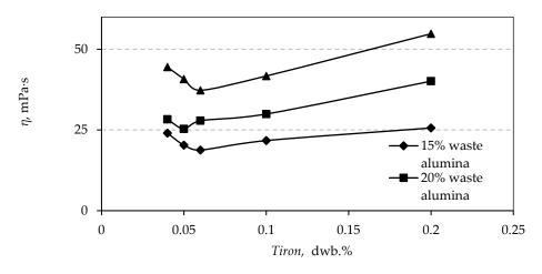
Figure 1. Apparent viscosity of alumina 70 wt.% suspensions with three different amounts of waste alumina powder as a function of Tiron concentration (dwb.%).
