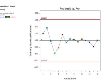
Figure A3. The plot of residuals versus the experimental run order.
