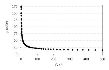
**Figure 4.** Plot of apparent viscosity ( $\eta$ ) versus increasing shearing rate ( $\gamma$ ) for 70 wt.% Al<sub>2</sub>O<sub>3</sub> water based suspension which contains 20 dwb.% of waste Al<sub>2</sub>O<sub>3</sub> powder, with optimal amounts of additives.
