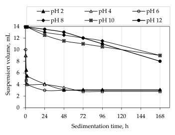
Figure 7. Sedimentation rate of water-based alumina suspensions with optimal composition after 168 h (7 days).
