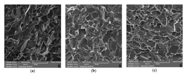
**Figure 3.** SEM images of alumina morphology sintered at 1550 °C with fixed weight ratios of waste alumina powder of 20 wt.%, 0.05 wt.% Tiron and 0.1 wt.% PVA and with varying amounts of magnesium aluminate spinel: (**a**) 0.2 wt.% MgAl<sub>2</sub>O<sub>4</sub>, (**b**) 0.6 wt.% MgAl<sub>2</sub>O<sub>4</sub> and (**c**) 1.0 wt.% MgAl<sub>2</sub>O<sub>4</sub> expressed on dry weight basis.
