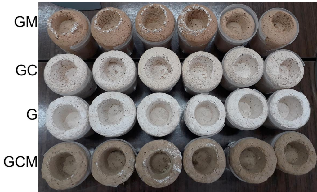
Figure S2. An efflorescence (white salt deposits) on or near the surface of pots, which were not subjected to neutralization process. Presented pots after 90 days of aging at ambient temperature and humidity. .
