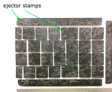
Figure 2. Preparation of SMC specimen out of the molded plate.
