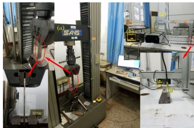
Figure 2. Metal magnetic memory detection system for stress evaluation. (a) CMT2502 testing machine. (b) EMS-2003. (c) Three-dimensional electrically controlled displacement system. (d) Two-channel pen sensor probe.
