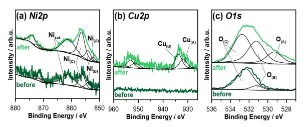
**Figure 9.** High-resolution XPS spectra recorded for blank Ni coating in (**a**) Ni2, (**b**) Cu2p, and (**c**) O1s peak binding energy range, before and after the exposure to 0.05 M NaCl.
