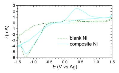
**Figure 3.** Cyclic voltammetry curves recorded in a blank Ni plating bath and suspension bath containing 2 g dm<sup>-3</sup> Ce<sub>2</sub>(MoO<sub>4</sub>)<sub>3</sub> 4.5H<sub>2</sub>O microflakes, at 70 °C on a rotating disk electrode with Pt tip (3 mm diameter), at 600 rpm.
