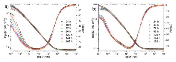
**Figure 7.** Bode representation of the impedance spectra recorded for (**a**) blank and (**b**) composite Ni coatings for 168 hours exposure in 0.05 M NaCl solution.
