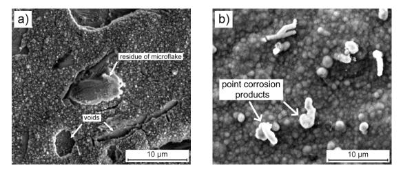
**Figure 11.** Surface morphology of (**a**) composite and (**b**) blank Ni coatings (deposited on the copper substrate at a current density of 6 mA cm<sup>-2</sup> at 70 °C for 1 h) after one-week exposure to 0.05 M NaCl solution.
