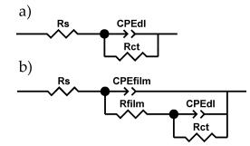
**Figure 8.** Electric equivalent circuits used for fitting the experimental spectra of (**a**) blank and (**b**) composite Ni coatings.
