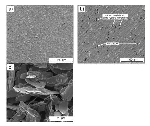
**Figure 1.** Surface morphology of (a) blank and (b) composite Ni coatings deposited on the copper substrate at a current density of 6 mA cm<sup>-2</sup> at 70 °C for 1 h, and (c) as-synthesized cerium molybdenum oxide hydrate microflakes for comparison. Pictures were recorded in a SE mode of SEM.
