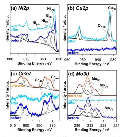
**Figure 10.** High-resolution XPS spectra recorded for composite Ni coating in (**a**) Ni2p, (**b**) Cu2p, (**c**) Ce3d, and (**d**) Mo3d peak binding energy range, before and after the exposure to 0.05 M NaCl. The chemistry of synthesized cerium molybdenum oxide hydrate powder used for electrodeposition is also shown in (**c**) Ce3d and (**d**) Mo3d spectra ("reference" spectra).
