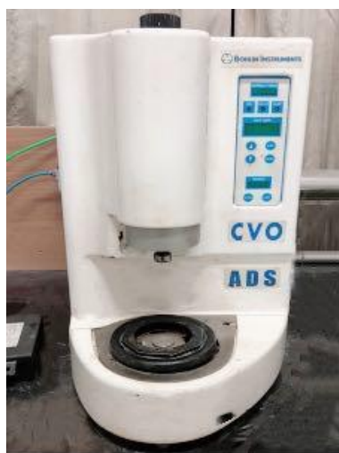
Figure 4. Dynamic shear rheometer.
