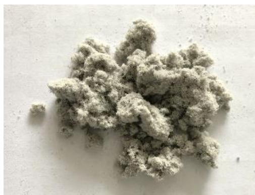
Figure 2. Macro image of lignin fiber.
