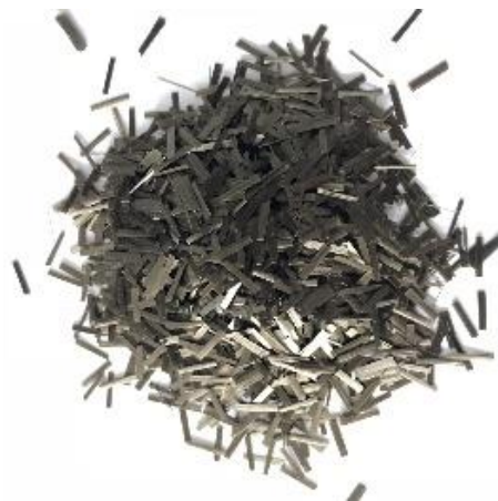
Figure 1. Macro image of basalt fiber.
