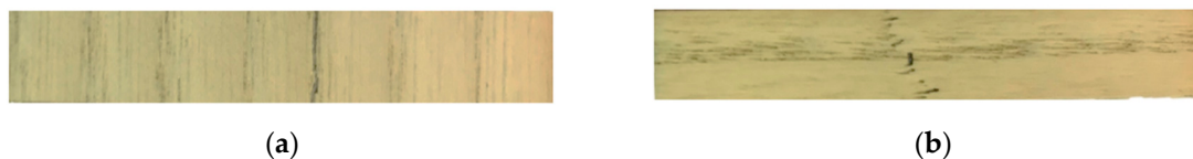
Figure 3. Perpendicular (a) and longitudinal tensile samples (b) of VL with failure.
