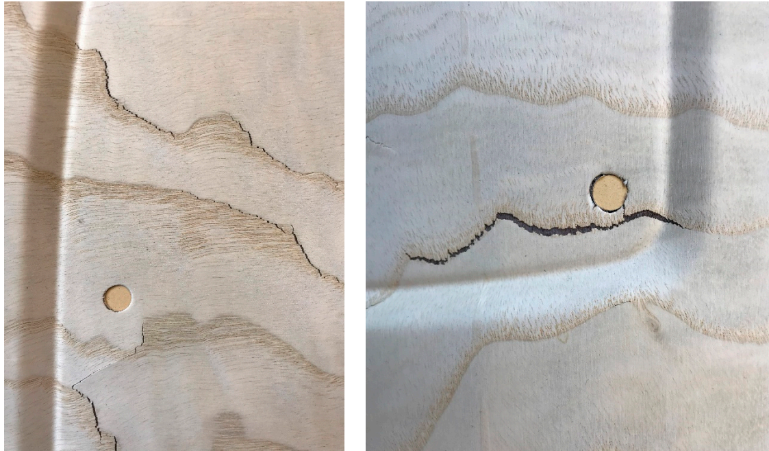
Figure 1. Two examples of veneer laminate sheets after forming into a trim part geometry, which show characteristic fracture along earlywood (EW) zones.
