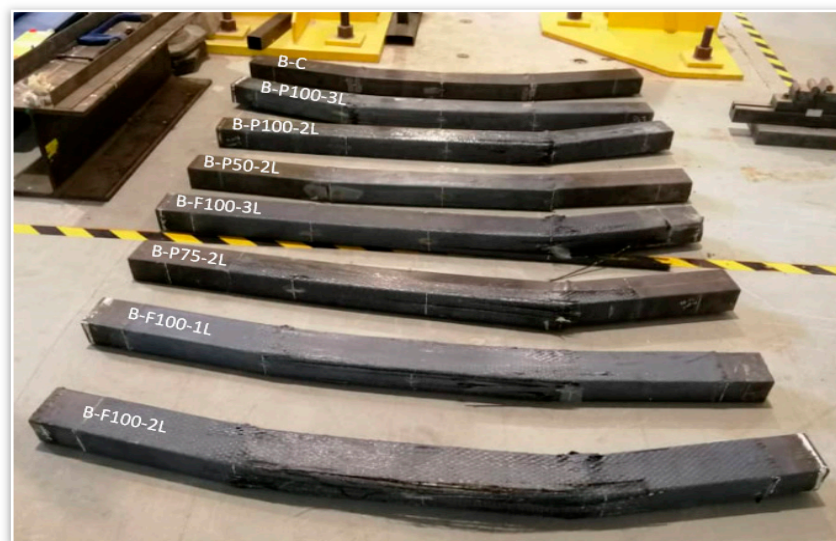
Figure 14. Failure modes of all tested HPCFDST samples.
