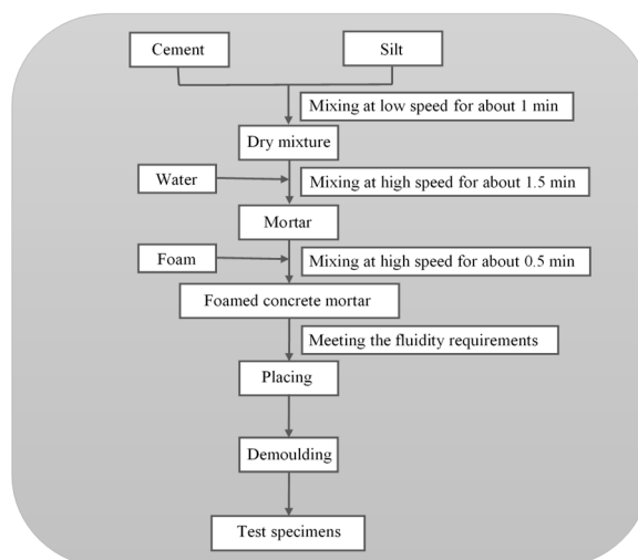
Figure 2. Procedure of preparation of foamed concrete.
