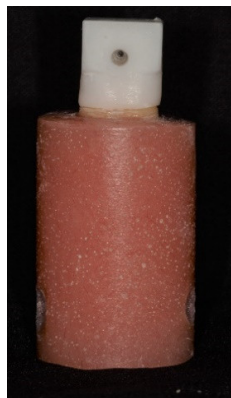
Figure 1. Zirconium oxide coping showing the design of the occlusal surface to enable removal post-cementation.
