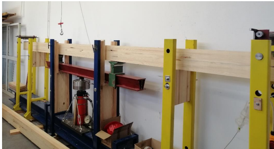
Figure 3. Test stand for the evaluations of the bending strength and modulus of elasticity.
