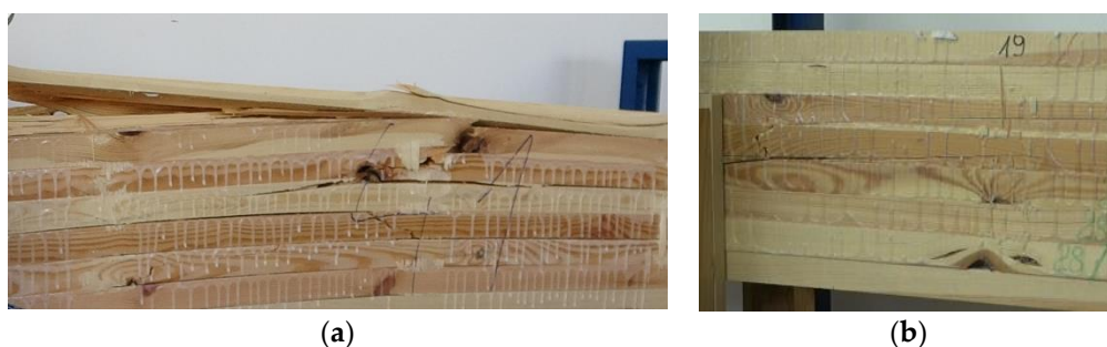
Figure 7. Beam failure images: (a) GL24c—MOR(MOR 12% )—48.5(43.4) \text{N/mm}^2 —the strongest in the group, (b) GL28c—MOR(MOR 12% )—30.4(25.8) \text{N/mm}^2 —the weakest in the group.
