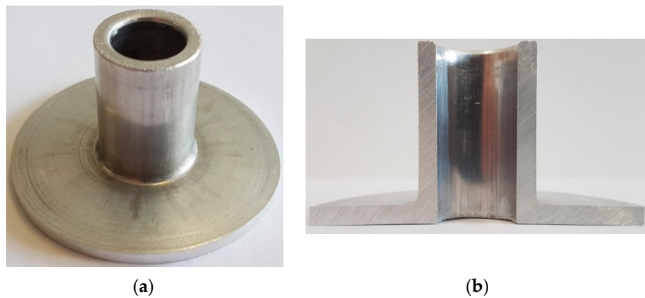
Figure 5. Hollow part with a 56 mm diameter flange: (a) perspective view, (b) axial section.
