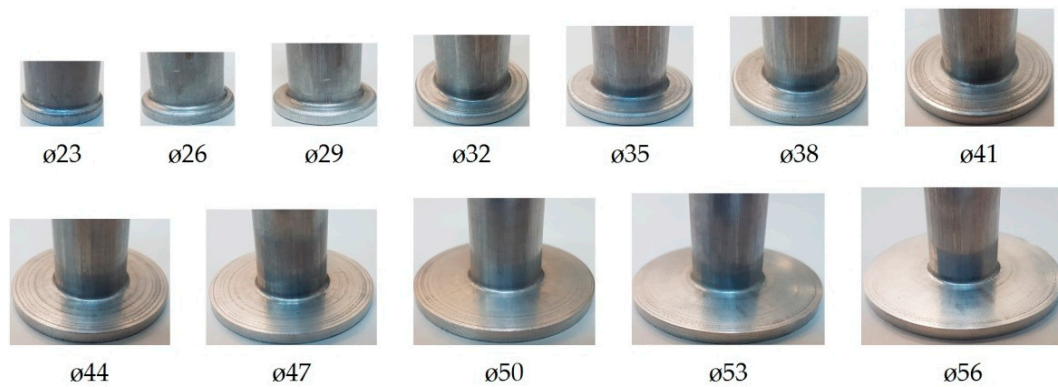
Figure 4. Changes in flange shape in incremental radial extrusion.
