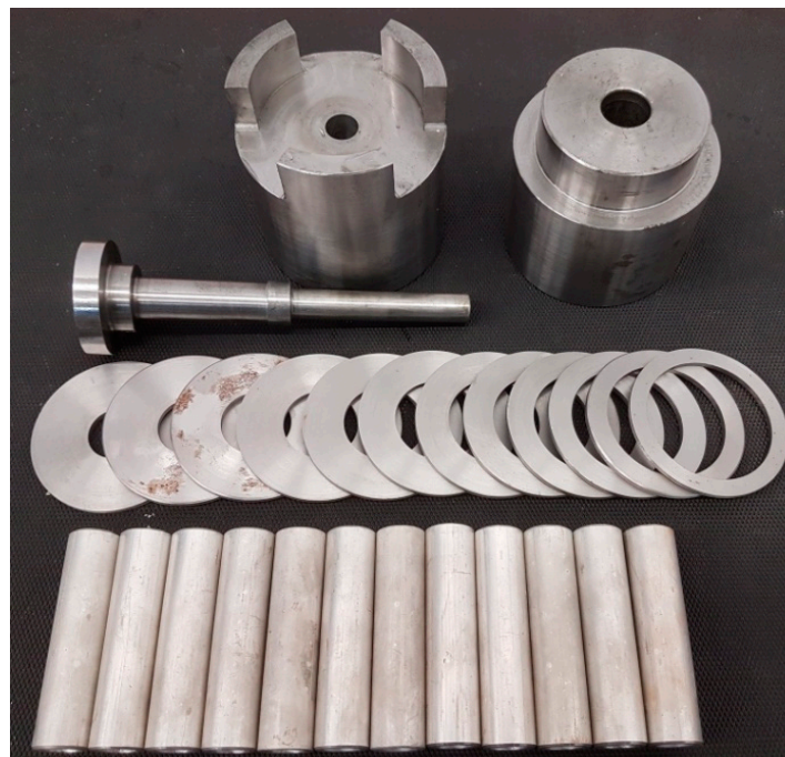
Figure 2. Tools and billets used in the incremental radial extrusion of the flange.
