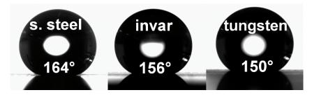
Figure 8. The wettability measurements of laser processed samples after vacuum treatment.
