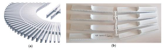
**Figure 1.** PP plastic ribs that are the object of the case study. (a) Assembly of a chain of ribs into a swimming pool water sink cage. The assembly can form a straight line or follow curves (picture courtesy of Fluidra group). (b) A set of 8 ribs resulting from an injection operation.
