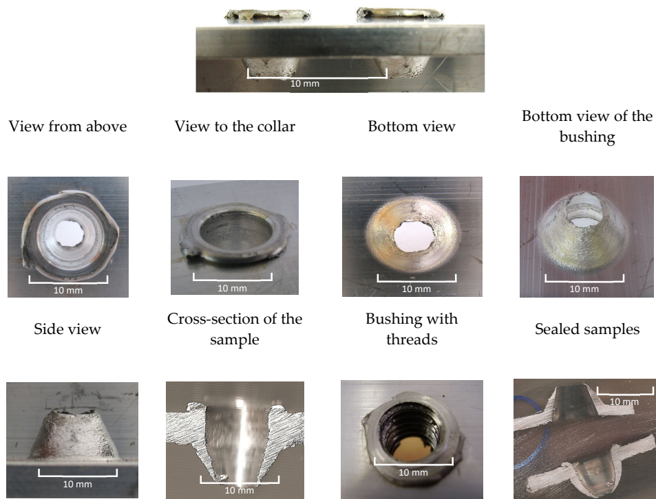
Figure 6. Visual evaluation of collars and bushings from one layer of the AL alloy material—Al Mg Si.
