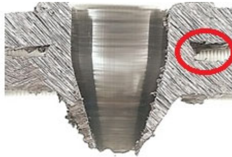
Figure 12. Place for SEM and EDS analysis: mixed part and initiation of the crack from inside the bushing.
