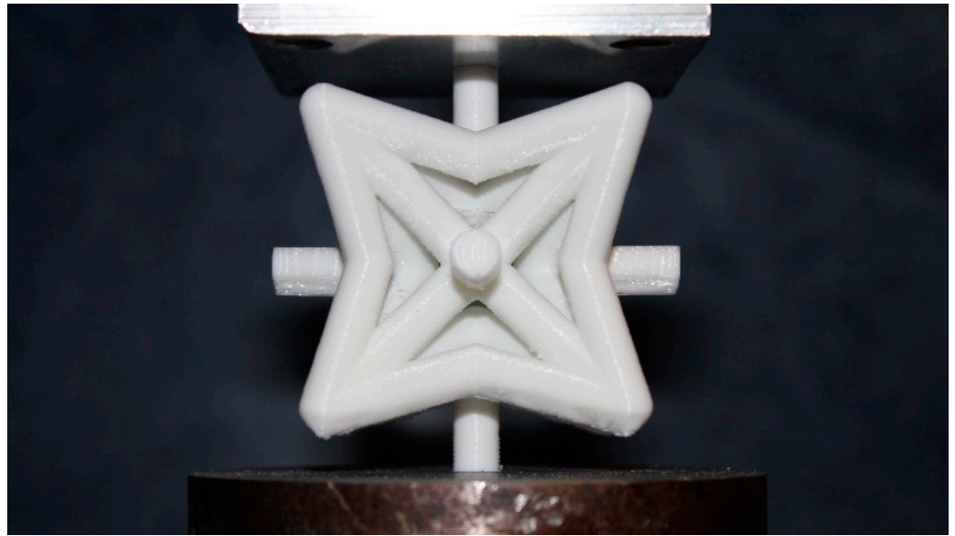
Figure 8. An additively manufactured specimen with \mu = 0.25 under loading test.
