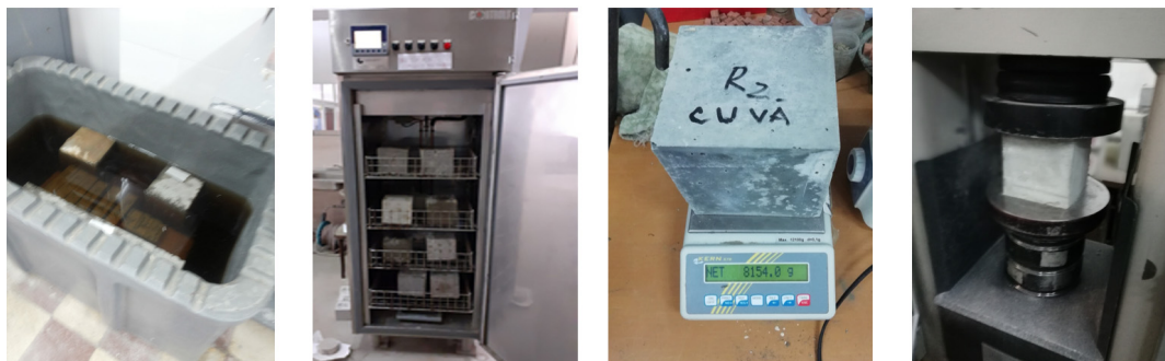
Figure 1. Control specimens kept in water and specimens underwent the freeze–thaw test (150 mm × 150 mm × 150 mm).
