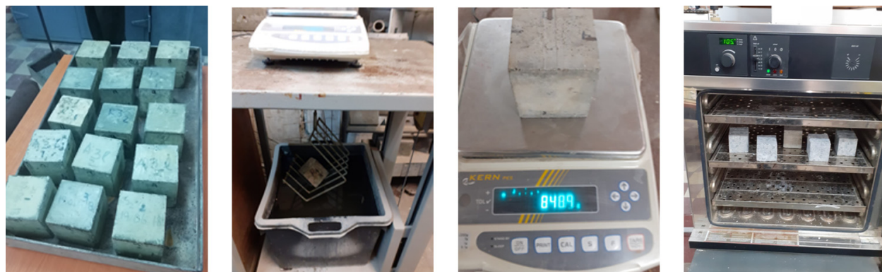
Figure 3. Hydrostatic weighing of cubes with 71 mm side.
