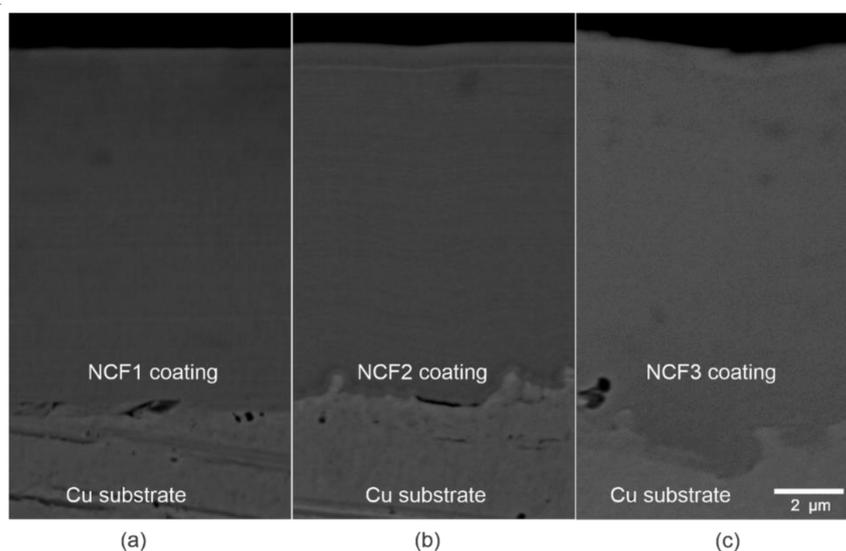
**Figure 5.** Cross-sections of the Ni-Co-Fe coatings: (a) NCF1, (b) NCF2, (c) NCF3, SEM BSE images.
