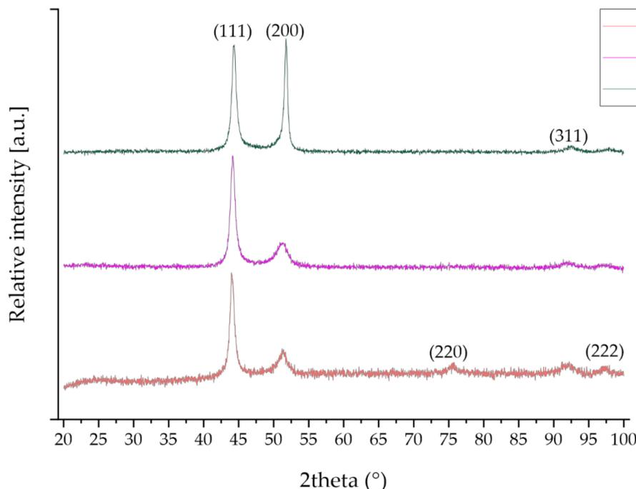
Figure 2. XRD spectra of ternary Ni-Co-Fe coatings.
