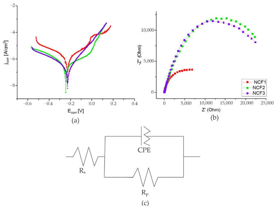
**Figure 9.** (a) Polarization curves, (b) Nyquist plots of ternary Ni-Co-Fe curves, (c) Randles equivalent circuit ( $R_s$ —solution resistance,  $R_p$ —charge transfer resistance, CPE—double layer capacity) obtained for Ni-Co-Fe coatings.
