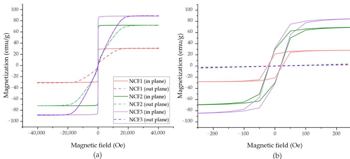
**Figure 8.** (a) Magnetic hysteresis loops measured at room temperature for ternary Ni-Co-Fe alloys shown in the full range and (b) at the small field area, in-plane (solid line), and out-of-plane (dash line) geometry.
