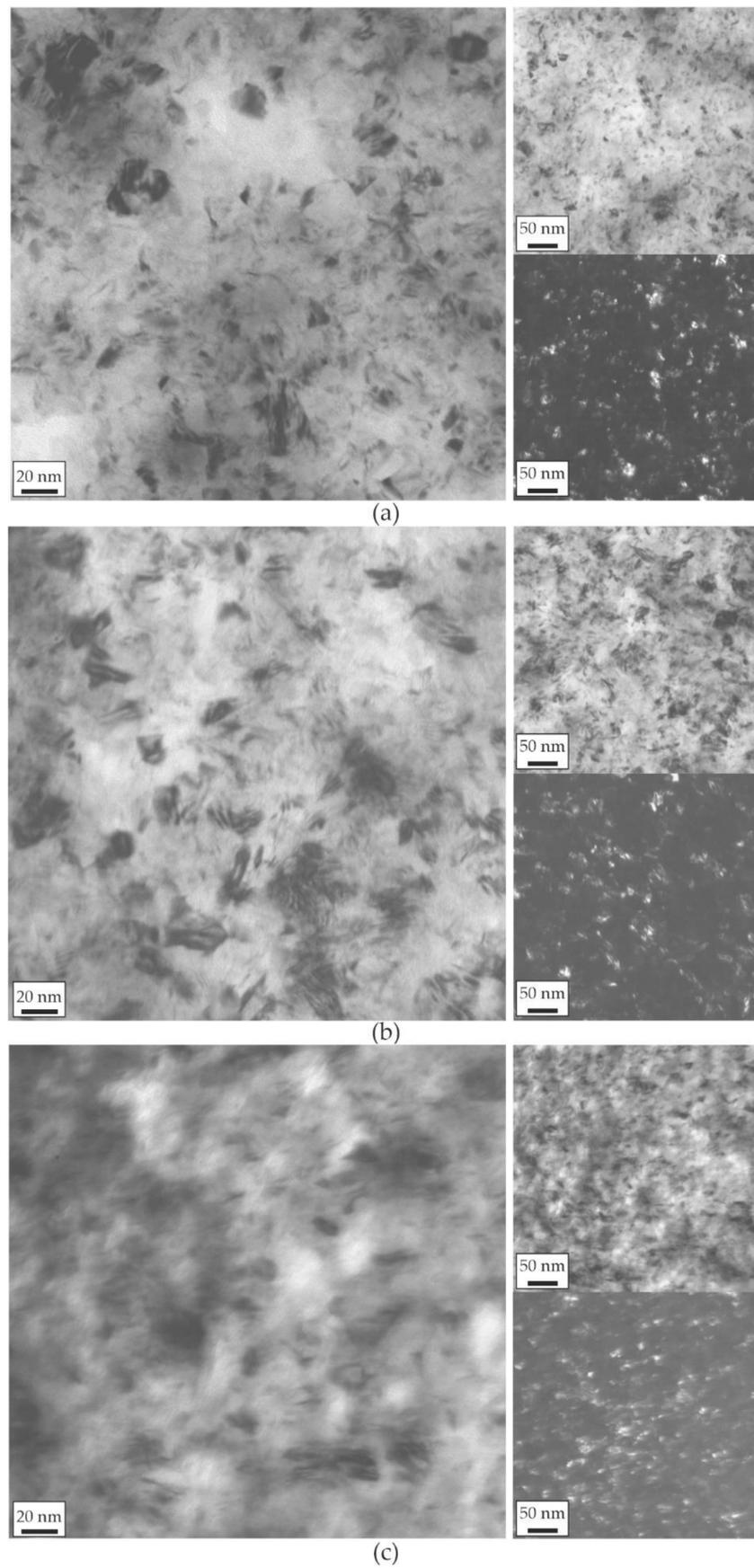
**Figure 6.** TEM bright-field images of (a) NCF1, (b) NCF2, and (c) NCF3 coatings and at the right the pairs of the lower magnification bright- and dark-field images taken in (111) ring of the  $\gamma$  phase.
