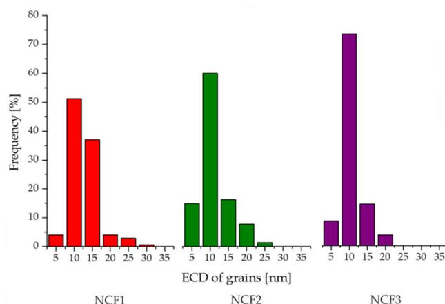
Figure 7. Grain size distribution in NCF1, NCF2, and NCF3 coatings.
