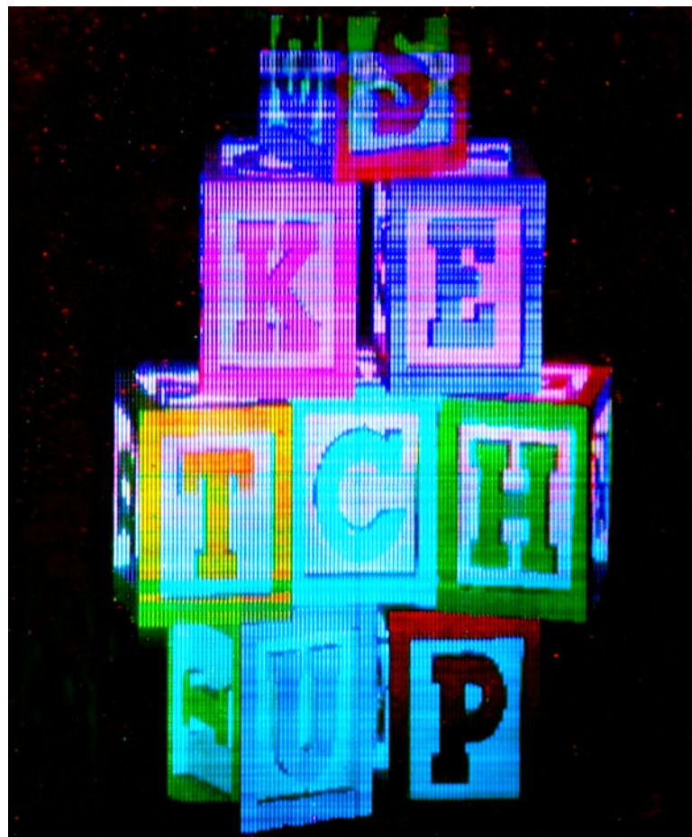
Figure 9. Picture of a full color (red, green, and blue) holographic stereogram recorded in photorefractive polymer by taking advantage of the symmetry and polarization of the recording beams, as described in the text. The material composition was TPD:CAAN/FDCST:BBP:PCBP (56.2:33.7:9.8:0.2).
