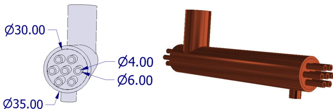
Figure 2. General view of the shell-and-tube exchanger.
