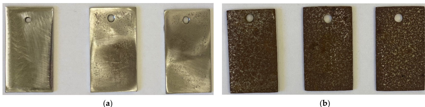
Figure 4. Steel samples after weathering tests for 9 months: chamber treatment with CIN vapors (a); without chamber treatment (b).
