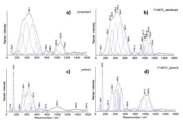
**Figure 9.** Representative Raman spectra recorded on the *cloisonné* enamels of the ewer (baseline subtracted): turquoise (a), dark blue (b), yellow (c), and green (d). Gaussian and Lorentzian components used to separate the contribution of the crystalline pigment from that of the glassy matrix are shown.
