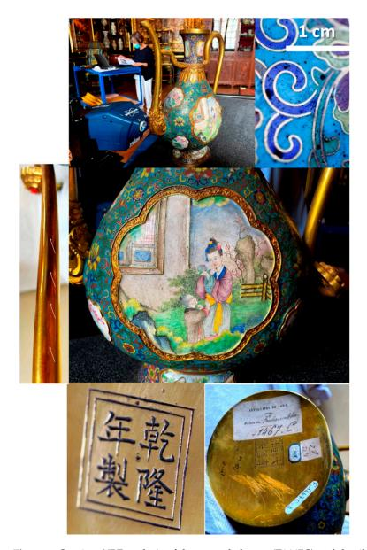
**Figure 1.** On-site pXRF analysis of the enameled ewer (F1467C) and details of the décor (*cloisonné* and painted enamels); the bottom face exhibits an engraved Qianlong reign mark (bottom left, basin: *Qian long nian zhi*; right, ewer; *Da qing Qian long nian zhi*). Note the welding traces along the spout (arrows).
