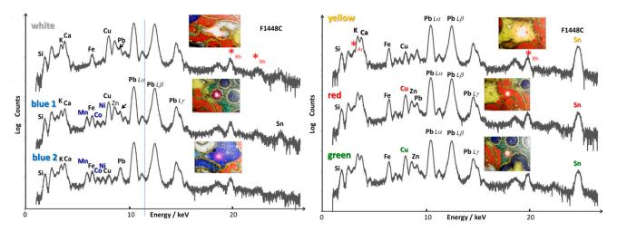
**Figure 5.** Representative pXRF spectra recorded on the different colored *cloisonné* enamels of the incense burner (white, blue, yellow, red and green areas). Red stars (\*) indicate the contribution of the instrument (Rh peaks).
