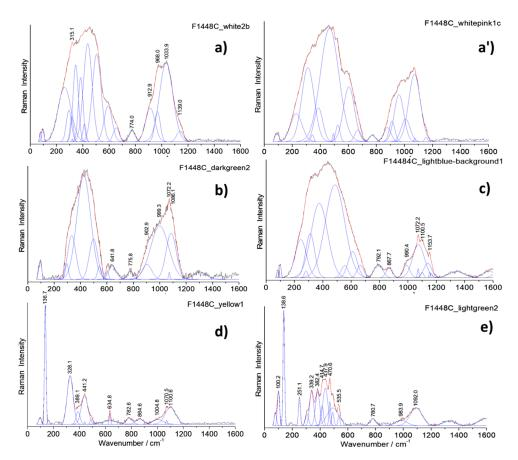
**Figure 8.** Representative Raman spectra recorded on the *cloisonné* enamels of the incense burner (baseline subtracted): white (a), white-pink (a'), dark green (b), turquoise (c), yellow (d) and light green (e) areas. Gaussian and Lorentzian components used to separate the contribution of the crystalline pigment from that of the glassy matrix are shown.
