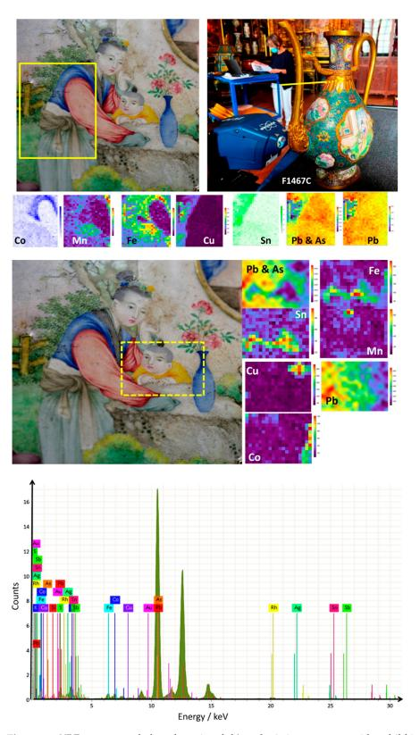
**Figure 7.** pXRF maps recorded on the painted décor depicting a woman with a child in the garden. The two mapped areas are delimited with a yellow line. The optical pixel image and corresponding distribution of elements (Co, Mn, Fe, Pb, Cu, Sn and Pb + As) are shown. An example of an XRF spectrum recorded on the darkest blue area of the woman's vest in the painted décor.
