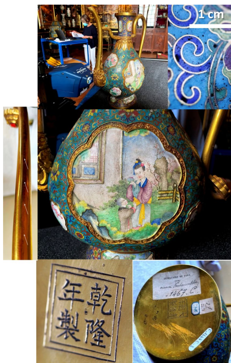
Figure 1. On-site pXRF analysis of the enameled ewer (F1467C) and details of the décor ( cloisonné and painted enamels); the bottom face exhibits an engraved Qianlong reign mark (bottom left, basin: Qian long nian zhi ; right, ewer; Da qing Qian long nian zhi ). Note the welding traces along the spout (arrows).3.2.2. Ewer (3rd quarter of 18th century, Qianlong mark).
