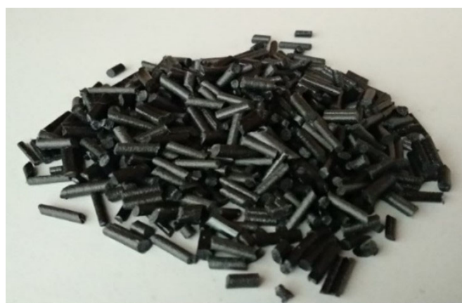
Figure 3. rCF/PLA pellets after the mixing and palletizing process.
