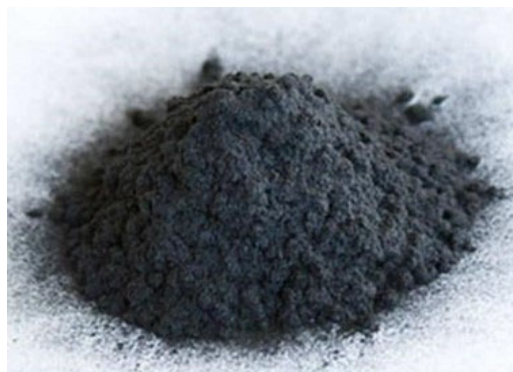
Figure 1. rCF recovered from a pyrolysis process.
