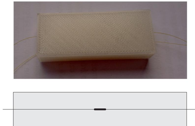
**Figure 3.** A photograph and cross-section scheme of the PLA sample.
