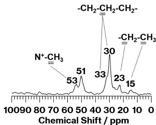
Figure 3.  $^{13}\text{C}$  CP MAS NMR spectrum of C18TAC/MeO-Kaol\_Wash.
