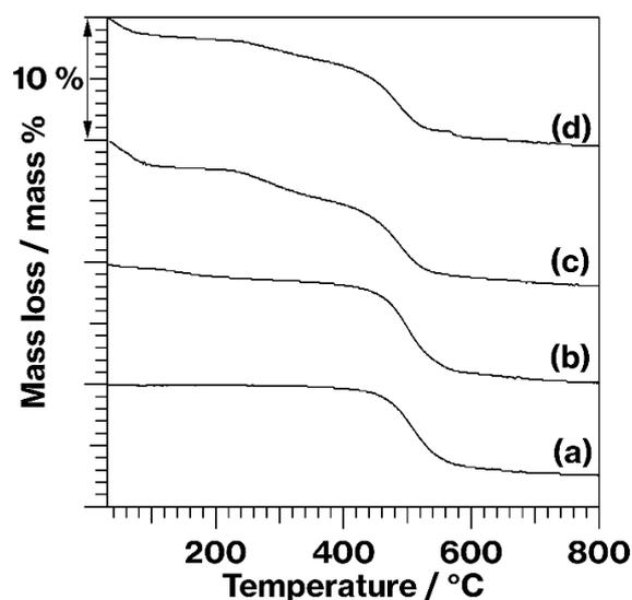
Figure 4. TG curves obtained from (a) kaolinite, (b) MeO-Kaol, (c) C18TAC/MeO-Kaol\_Wash, and (d) C18TAB/MeO-Kaol\_Wash.
