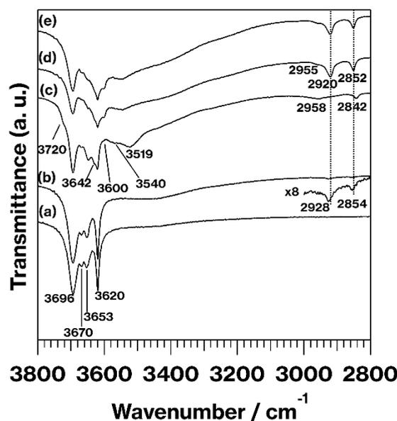
**Figure 2.** IR spectra in the range of 3800–2800  $\text{cm}^{-1}$  obtained from (a) kaolinite, (b) C18TAC/kaolinite\_Wash, (c) MeO-Kaol, (d) C18TAC/MeO-Kaol\_Wash, and (e) C18TAB/MeO-Kaol\_Wash.
