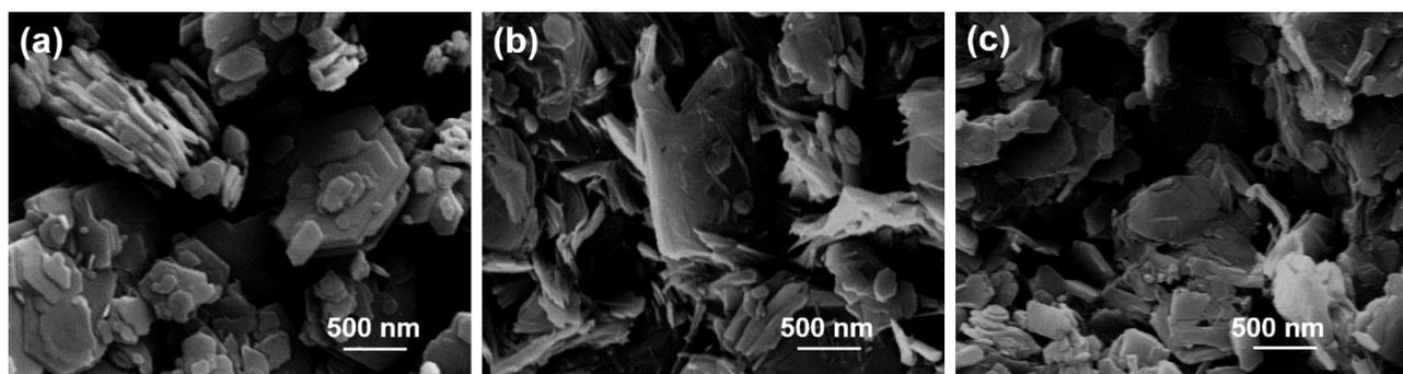
**Figure 5.** FE-SEM images of (a) MeO-Kaol, (b) C18TAC/MeO-Kaol\_Wash, and (c) C18TAB/MeO-Kaol\_Wash.
