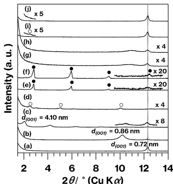
**Figure 1.** XRD patterns obtained from (a) kaolinite, (b) MeO-Kaol, (c) C18TAC/MeO-Kaol, (d) C18TAC, (e) C18TAB/MeO-Kaol, (f) C18TAB, (g) C18TAC/MeO-Kaol\_Wash, (h) C18TAB/MeO-Kaol\_Wash, (i) C18TAC/kaolinite, and (j) C18TAC/kaolinite\_Wash. Reflections due to C18TAC and C18TAB are marked as open and closed circles, respectively. For (c), (e), (f), (i), and (j), adequately enlarged patterns in some  $2\theta$  ranges are shown above each original pattern.
