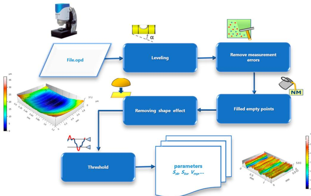
Figure 6. Methodology for data analysis of surface topography.
