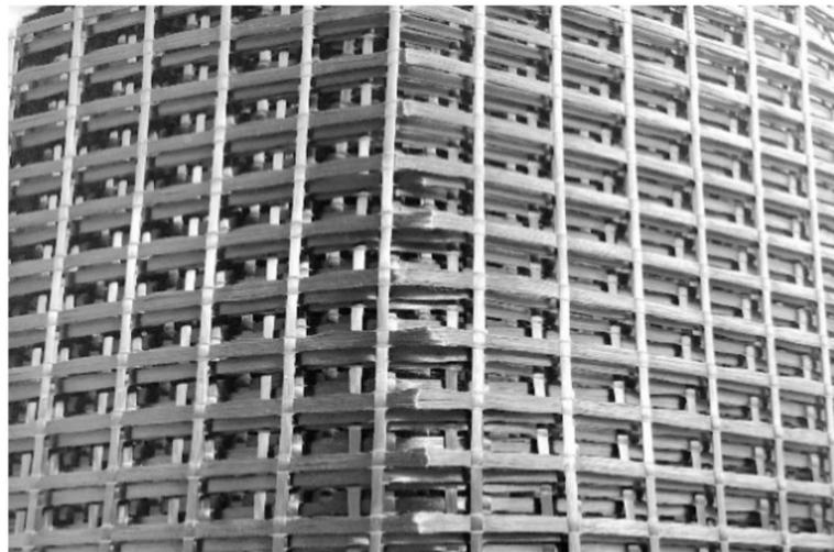
**Figure 9.** Damage in CF textiles due to transport.
