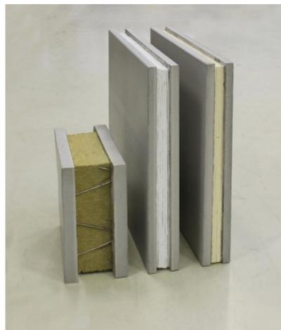
**Figure 5.** Comparison of a conventional reinforced concrete wall element (left) with two CRC wall elements with different aerogel insulation (middle, right).
