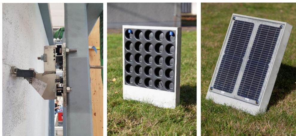
**Figure 6.** Electrically activatable connection made of shape memory alloy (left); CRC panel with integrated photovoltaics, voids, and capillary system, taken from [44] (middle and right).
