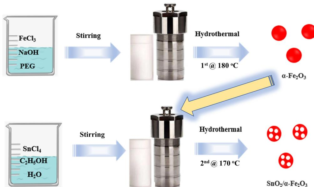
**Scheme 1.** Schematic diagram of the two-step synthesis process.
