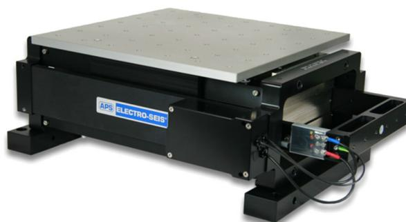
**Figure 4.** Uniaxial small-scale shaking table.
