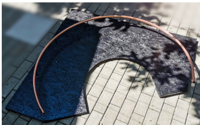
Figure 3. The rail fastened on the support board.
