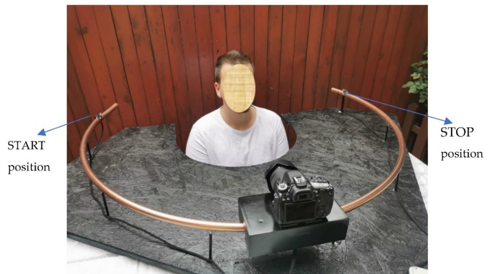
Figure 10. Process of human face scanning—between START and STOP positions.
