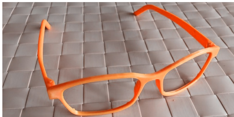
Figure 15. Result—3D-printed spectacles frames.
