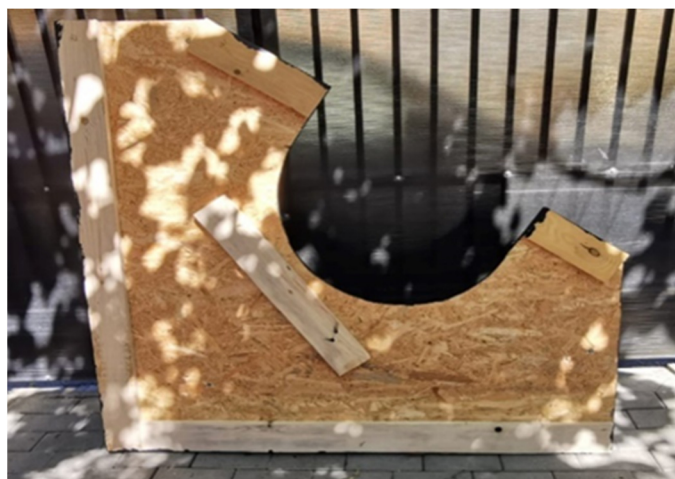
Figure 2. Rigid support manufactured from OSB board.
