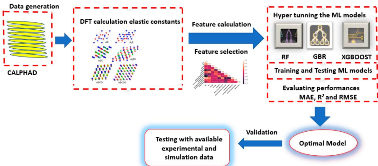
**Figure 2.** Graphic representation of the workflow process of the current study.
