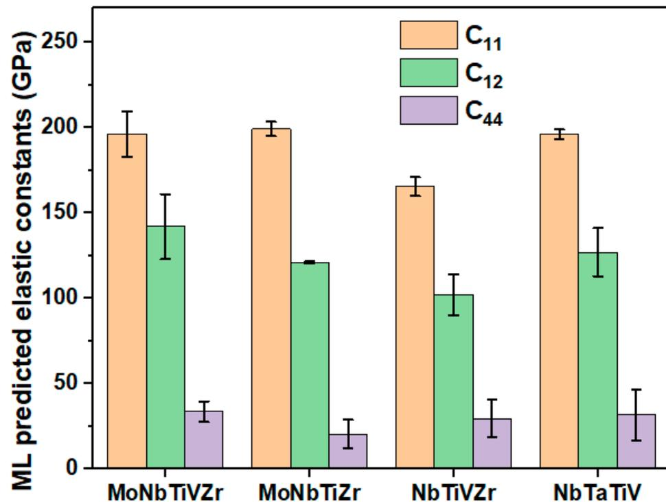
**Figure 6.** Elastic constants ( $C_{11}$ ,  $C_{12}$ , and  $C_{44}$  are in unit GPa) for MoNbTiVZr, MoNbTiZr, NbTiVZr, and NbTaTiV refractory alloys predicted by the GBR model. The error bar shows how far the elastic constant value has deviated from its original value.
