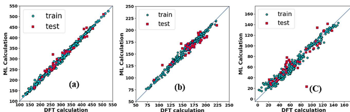
**Figure 5.** ML-predicted elastic constants of (a) C<sub>11</sub>, (b) C<sub>12</sub>, and (c) C<sub>44</sub>, as a function of DFT-predicted elastic constant during training and testing datasets.
