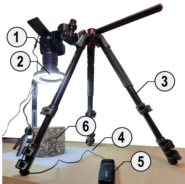
Figure 2. Test stand with DSLR camera (1), light source (2), tripod (3), uniform background (4), intervalometer (5) and tested specimen (6).
