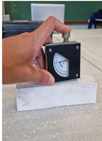
**Figure 3.** Shore C durometer test.
