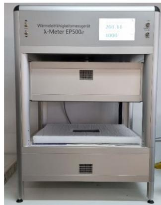
**Figure 9.**  $\lambda$ -meter machine setup.
