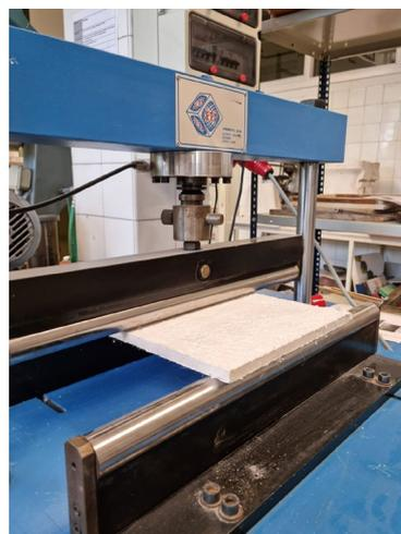
**Figure 2.** Bending test machine by Proeti, S.A. in Madrid.
