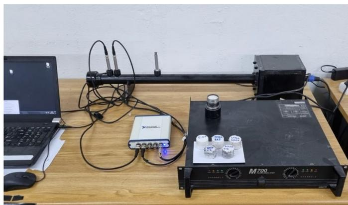
Figure 10. Impedance tube used.
