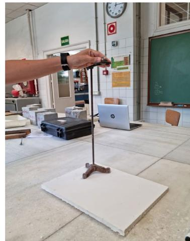
**Figure 4.** Surface hardness impact test.
