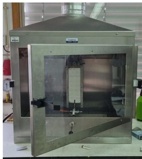
**Figure 13.** Fire ignitability test machine.
