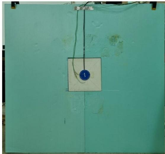
**Figure 6.** Sample placed in XPS frame.
