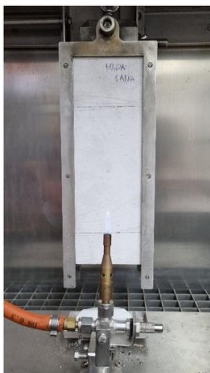
**Figure 22.** Ignitability test machine set up (UNE-EN-11925:1).
