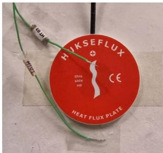
**Figure 7.** Thermocouple and heat flux meter setup.
