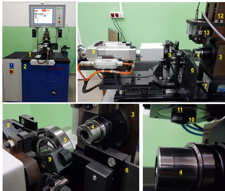
**Figure 1.** Laboratory rig for dynamic tests of bearings. The laboratory system is located at the Polish Bearings Factory in Krasnik.
